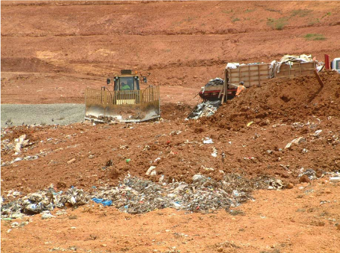
Cat 826 G operating at the tip face with daily cover over the waste
