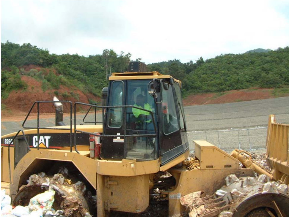
Caterpillar 826 G Landfill Compactor Weighing 36 tonnes
